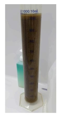
Acrylamide-based flocculants and chitosan were applied to wastewater exiting the drum-filter of a RAS, with the back-wash function. Effluents produced in salmon smolts (freshwater) and and seabass (seawater) were treated in the experiments. Flocculation was enhanced by the FP4 Portable Flocculation Tester, from Velp Scientifica.
