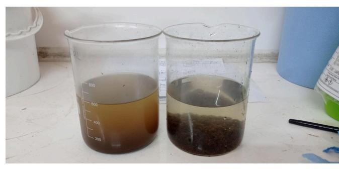
Sedimentation in non-flocculated wastewater (left) and flocculated wastewater (right), 5 minutes post flocculation.
