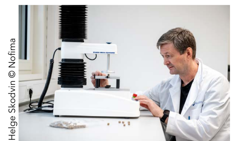
Fig 2. Pellet hardness testing at Nofima's Aqua Feed Technology Centre performed by Tor Andreas Samuelsen
