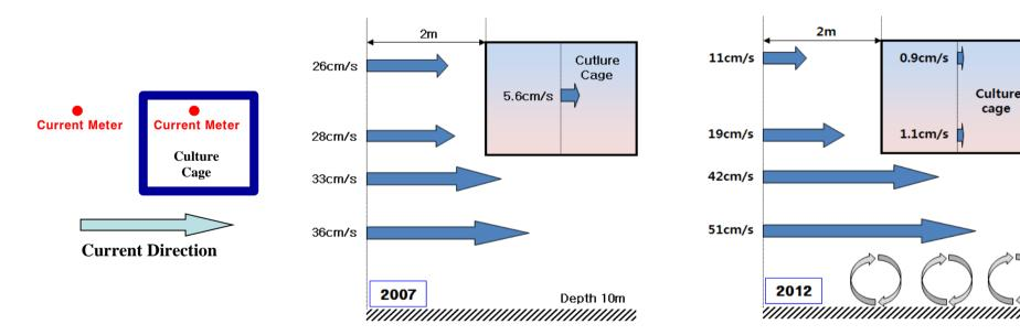
Schematic diagram showing plan view of hydrodynamic observation and vertical profile of current velocity inside and outside of abalone farm cage.
