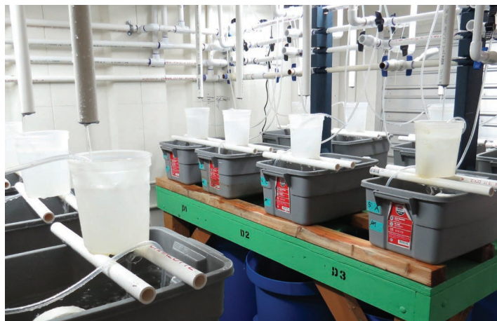
FIGURE 2. Experimental tanks used in temperature trials, with aerated head boxes and packed columns for degassing and aeration (Photo: James Barron).
