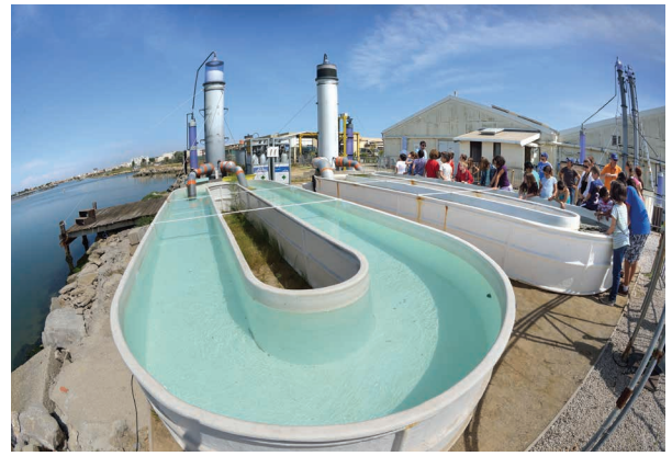
Microalgae research production tank at the Palavas research station of Ifremer. Photo: Olivier Dugornay, Ifremer.
