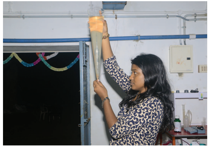
Checking the concentration of biofloc using an Imhoff cone.
