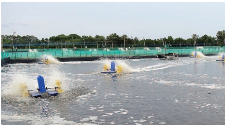
FIGURE 4. Intensive grow-out pond for shrimp in Indonesia using paddlewheel aerators.
